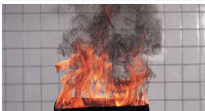
Test fire 5: liquid fire (n-heptane)
