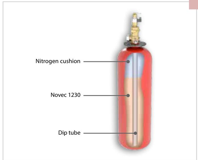
cushion in this first cylinder, the other cylinders are triggered pneumatically. At the same time the fire detection and extinguishing control panel triggers an audible and visual alarm, whereby persons present will be asked to leave the room.
