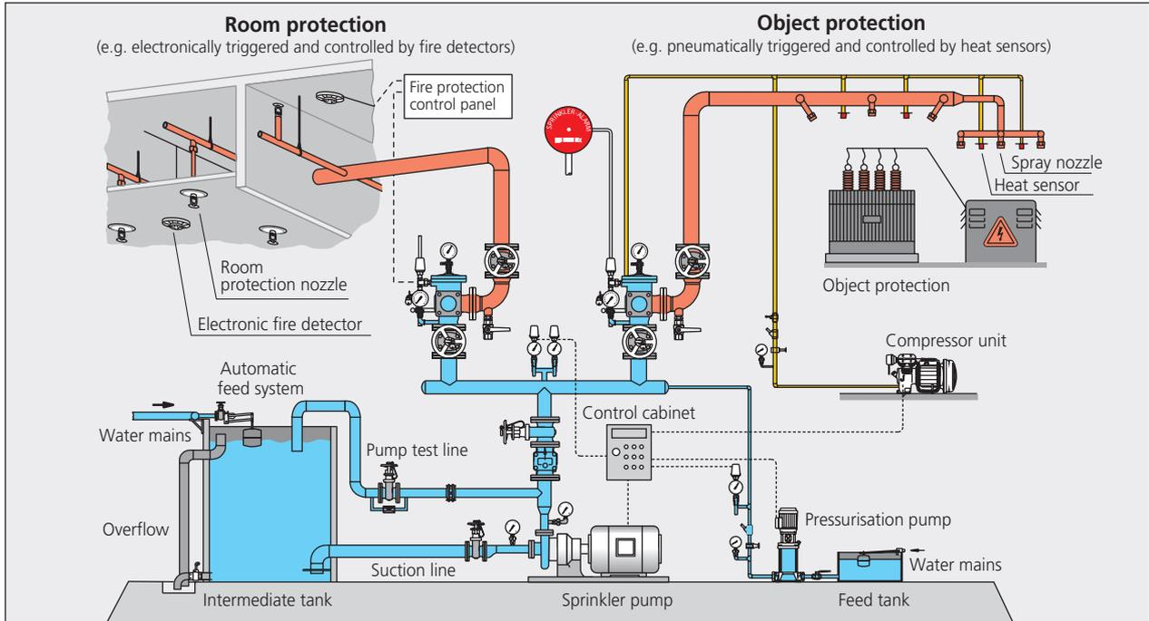
All sections of the building that are to be protected are equipped with a pipe system with open extinguishing nozzles. In ready mode, all piping up to the deluge valve is filled with water. The system includes fire detectors elements which, depending on the site conditions and the
